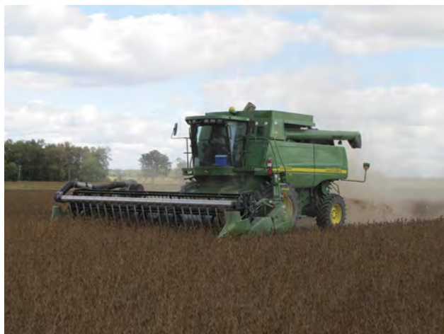
Photo 2–8. Combine with air reel to minimize losses.
